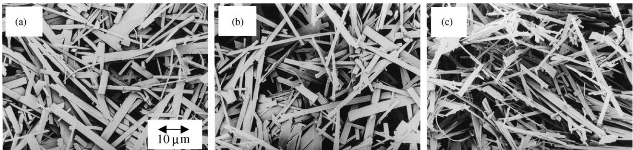
Fig. 6. SEM micrographs of the Ca-def HAp fibres synthesized from starting solutions with the Ca/P ratios of 1.00 (a), 1.40 (b) and 1.67 (c).
